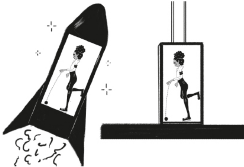
Figure 3.3. Gravity Girl experiments with gravity, as she is prone to do. From her point of view, when the rocket is being accelerated, the effect on the ball is the same as the effect of standing on Earth, where it is in the Earth's gravitational field. In both scenarios, the ball is accelerated downward relative to the rocket/elevator with an acceleration.
